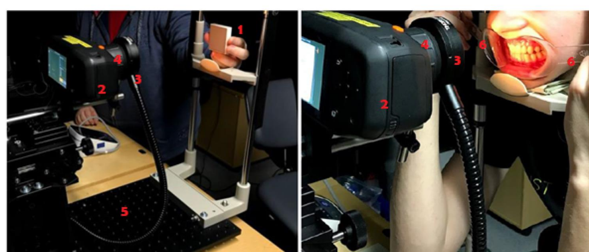
Figure 1. The process of hyperspectral imaging of oral cavity - front view. Left: neutral gray reference sample imaging. Right: imaging of oral cavity with lip retractor inserted. List of objects: 1 - neutral gray reference sample; 2 - hyperspectral camera; 3 - illumination ring; 4 - lens; 5 - construction; 6 - lip retractor
